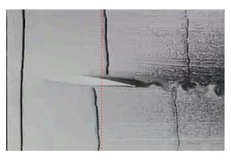
To sum up: the myth is that "...*air at the top has further to go. This means it goes faster..."* That is simply not true. Air above a flat airfoil is faster than the air below it, so it has nothing to do with the curvature.
